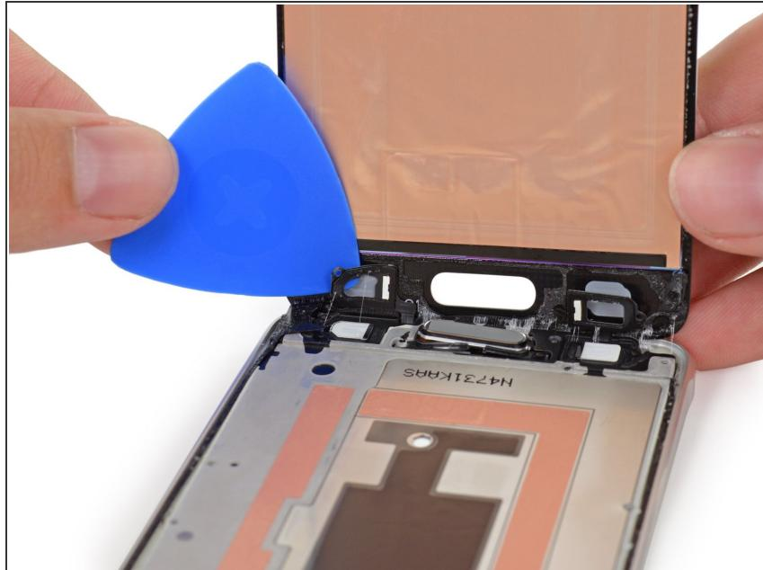
ⓘ Both the Samsung Galaxy S5 and iPhone 5s brought fingerprint scanning to the home button. And both did it fairly crudely, with a flimsy cable in the line of fire when opening the device.
