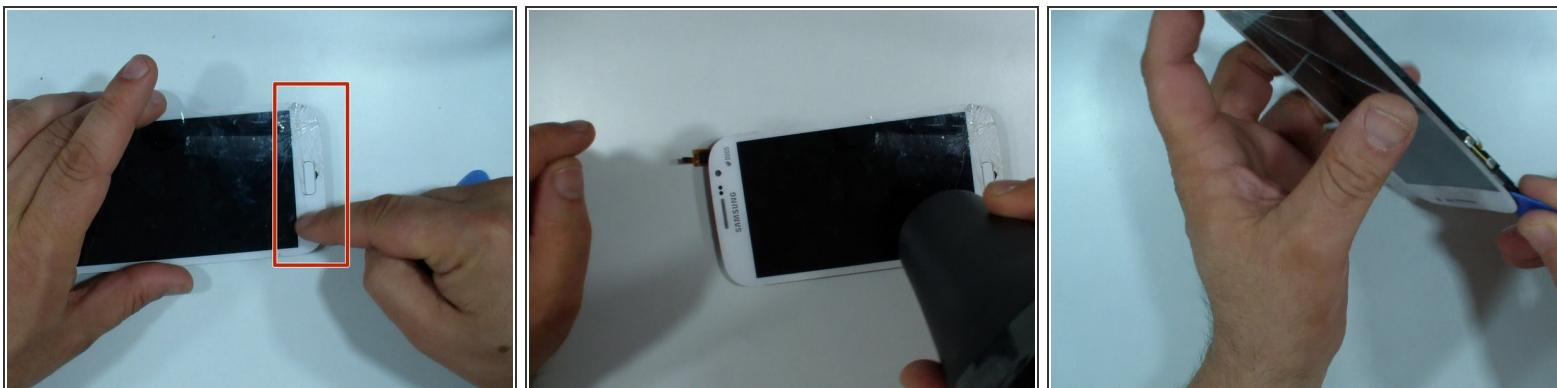
! At the bottom side, under the touch screen glass is the menu buttons flex cable. Be careful for it when you separating the glass from the frame.
