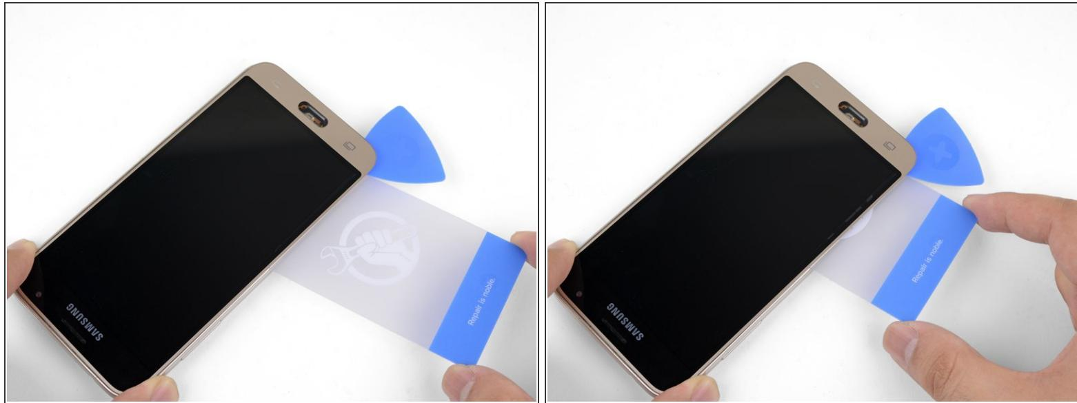
*(i)* The goal is to separate the LCD panel from the frame.
