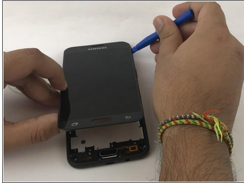
*(i)* Heating the surface of the screen will help with prying it off. It is recommended to use the iOpener.
