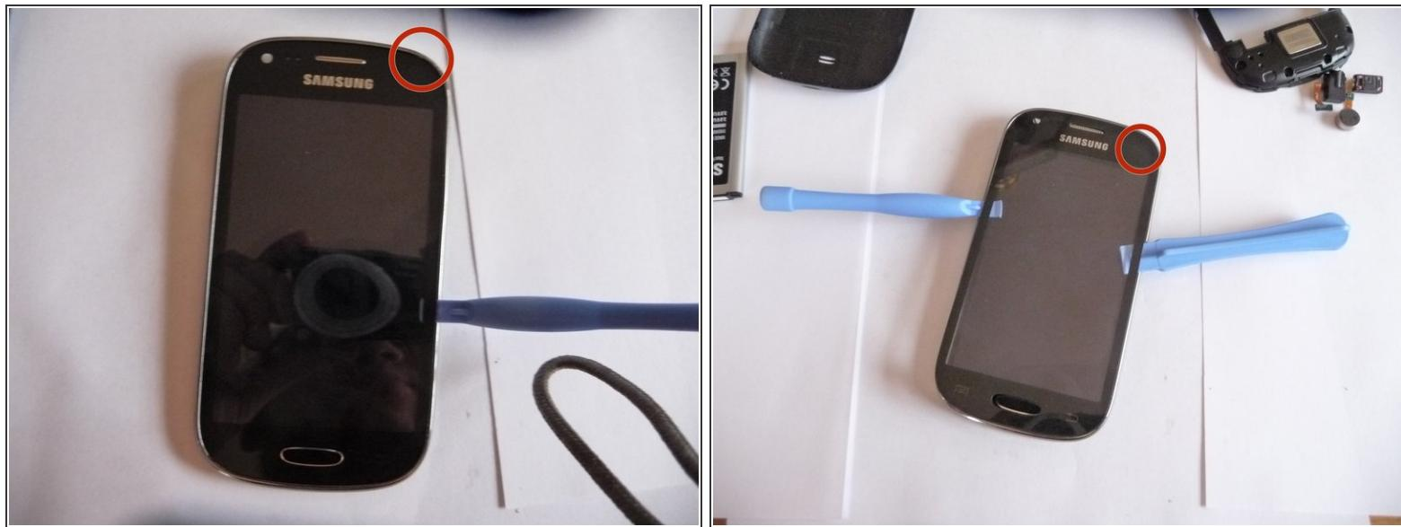
**⚠** The area highlighted in red is where the digitizer cable feeds through a slot in the frame. If you plan on reusing the digitizer be **very careful** when detaching the digitizer from this area or you may damage the cable.
