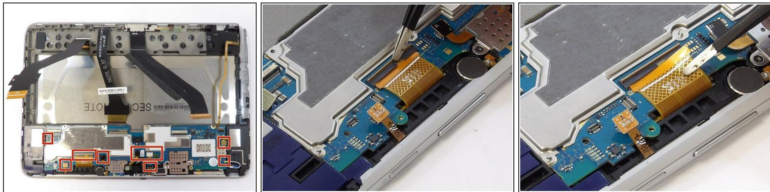
ⓘ Flip the tablet 180 degrees for this step so the motherboard is easier to access.
