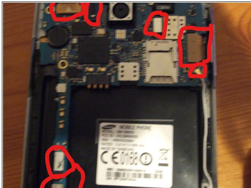
⚠ Be Careful !!! Take a look of the circuit board . It has 7 connections that you need to disconnect for the circuit board to be free .
