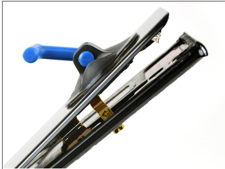
⚠ Both, the flex cable of the touchscreen and the display cable are threaded through the mid frame. The openings in the midframe are rather small and it can be a bit of a fumbling to pull them out.
