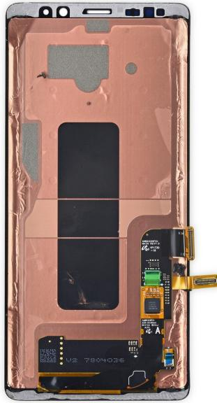
**⚠** Before installing a new display, it's very important to remove all traces of the old adhesive from the frame, while taking special care to remove any small glass fragments in case your display was broken.
