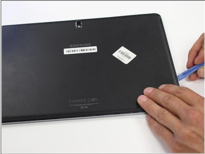
**i** Make sure the device is powered off before starting repair.
