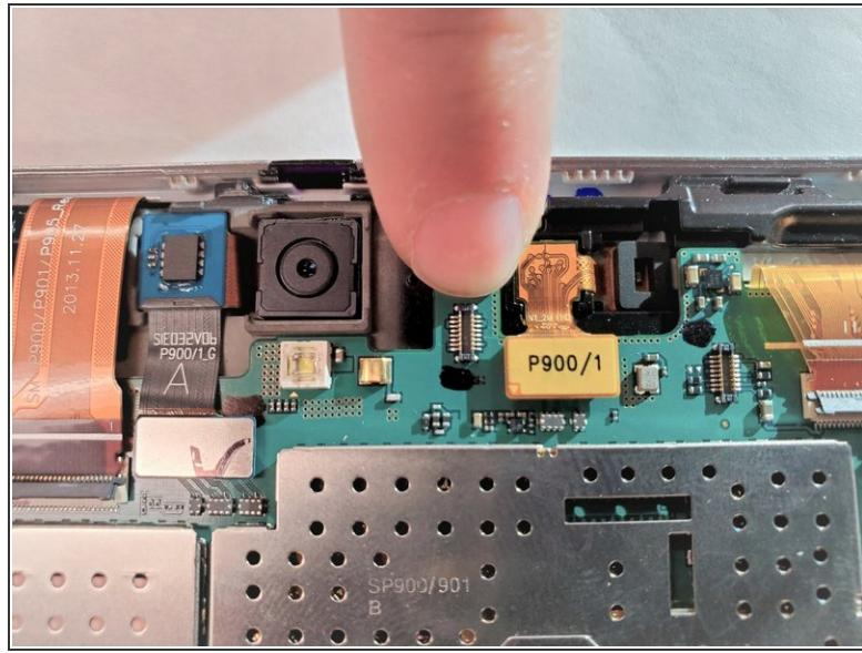
*(i)* The ambient light sensor is attached to the microphone. They come out together in one piece.
