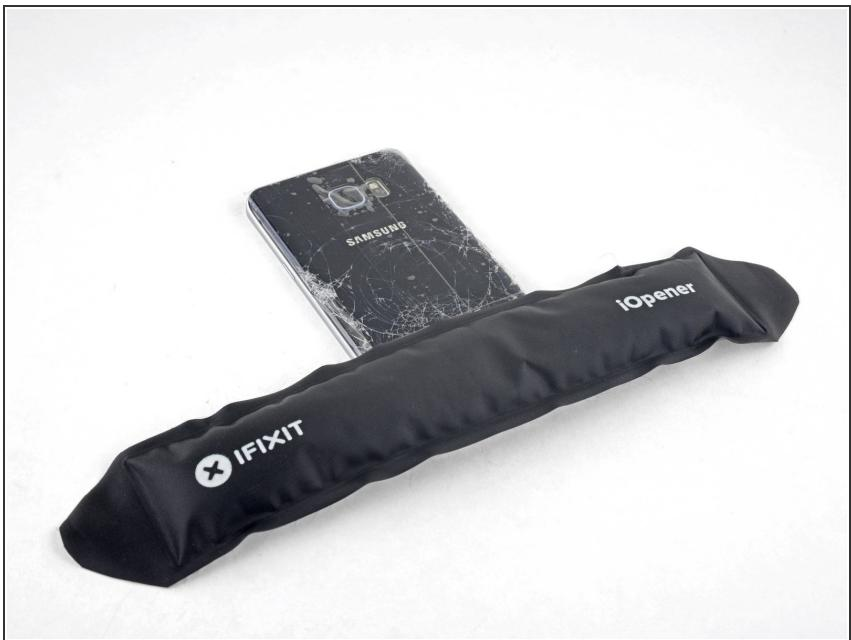
**i** If the glass back is cracked, [carefully tape over the entire surface with packing tape](#).
