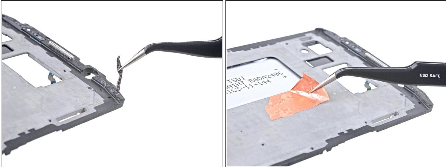
**⚠** Before installing a new display, it's very important to remove all traces of the old adhesive from the frame, while taking special care to remove any small glass fragments or other debris.
