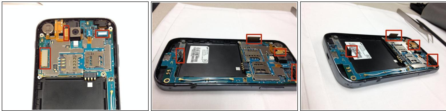
! The motherboard holds many delicate components, improper handling can result in the destruction of these components.
