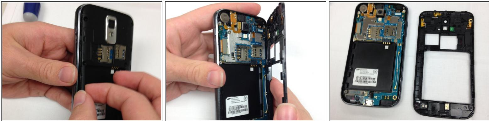
⚠ When removing the inner plate, place device on grounded surface or use anti static wrist band.
