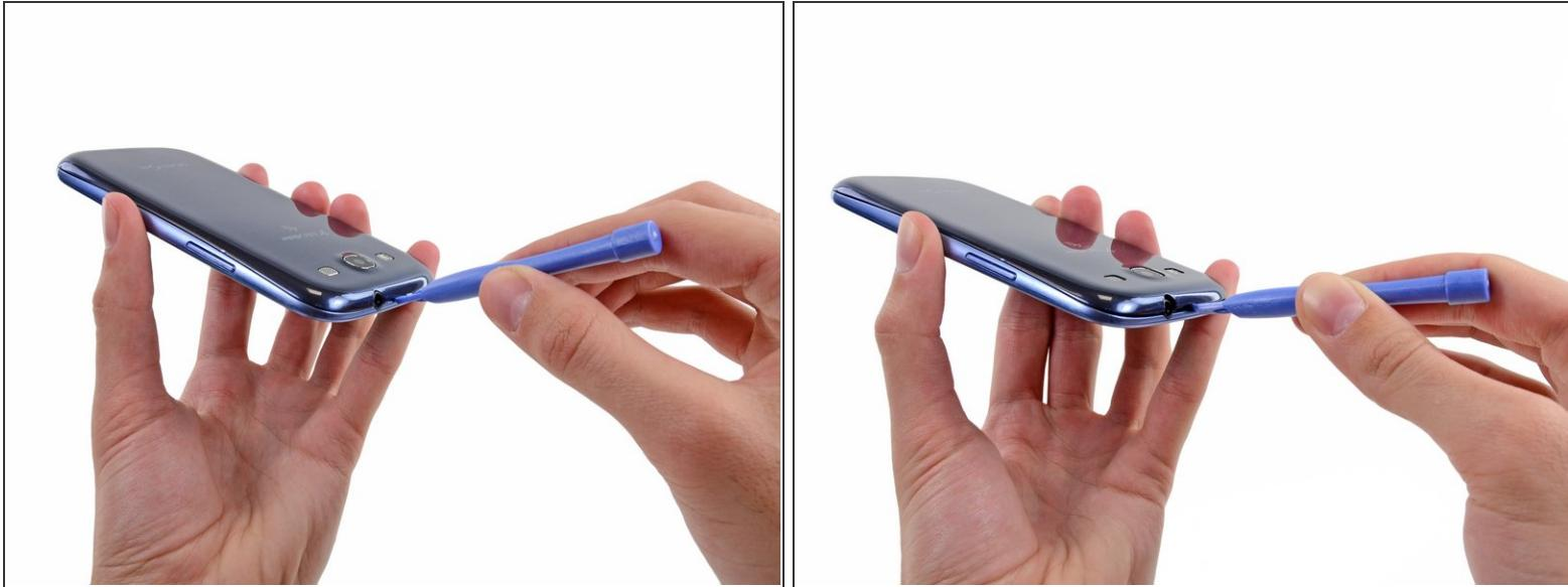
*(i)* The following four steps can be accomplished without a plastic opening tool. However, it's recommended to use a tool to best avoid breaking any clips along the perimeter of the rear case.
