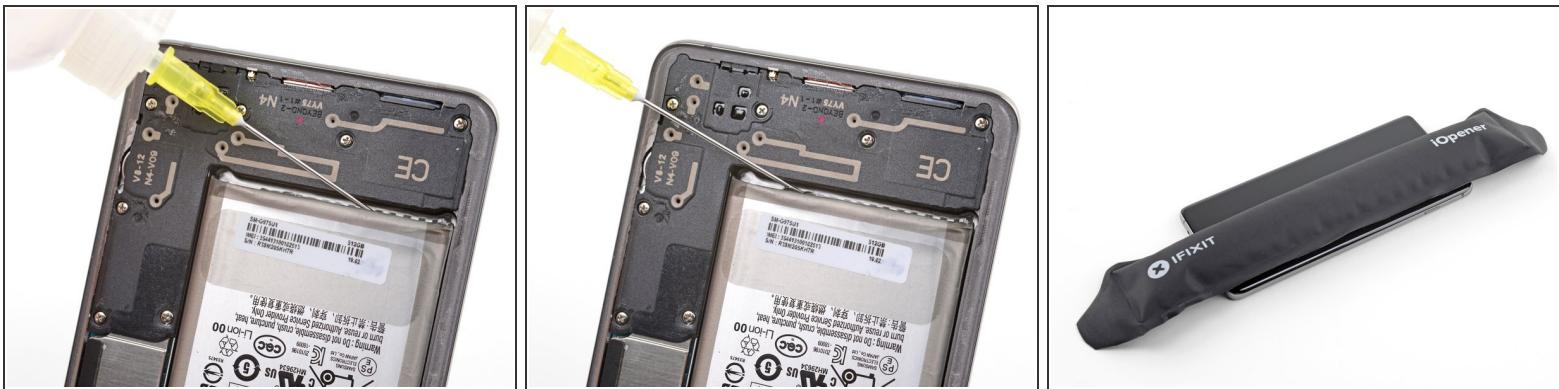
**i** Applying high concentration (over 90%) isopropyl alcohol to the battery will make the battery removal significantly easier.
