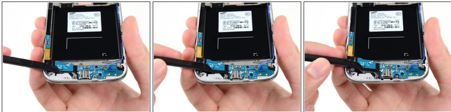
*(i)* The USB board is secured to the display assembly with light adhesive.
