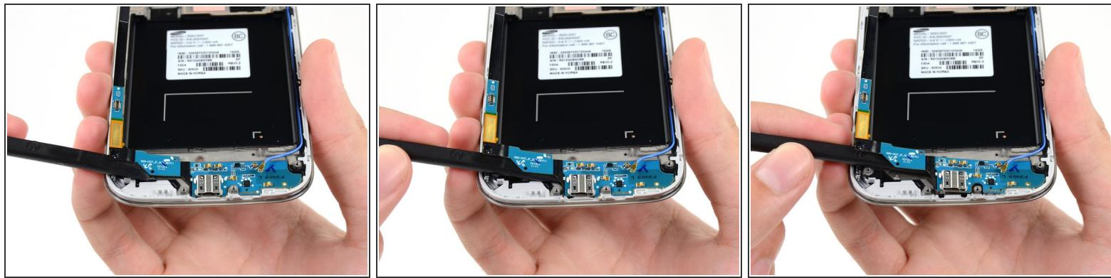
ⓘ The USB board is secured to the display assembly with light adhesive.
