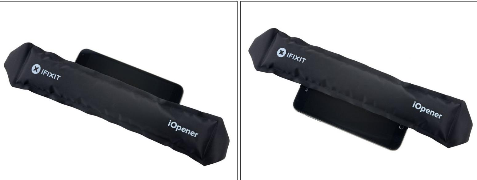
*(i)* In the following steps you will be using an iOpener to warm the adhesive affixing the display assembly to the rest of the phone. This will allow for a safer, easier screen removal. For proper iOpener use, follow our [iOpener heating guide](#), make sure to pay attention to all warnings.
