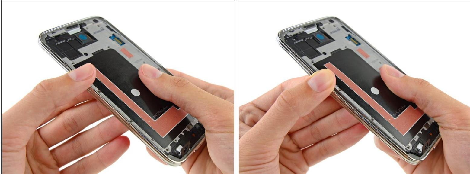
*(i)* The midframe is composed of two halves that encase the motherboard.
