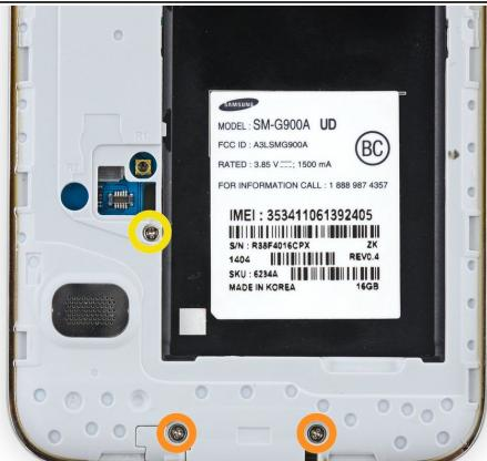
ⓘ Flip the phone over and remove the following screws from the battery side of the midframe:
