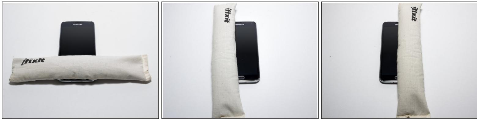
**⚠** Throughout this procedure you may need to reheat the iOpener. To prevent overheating the iOpener, always wait at least two minutes before microwaving again. Do not microwave the iOpener for more than one minute at a time.
