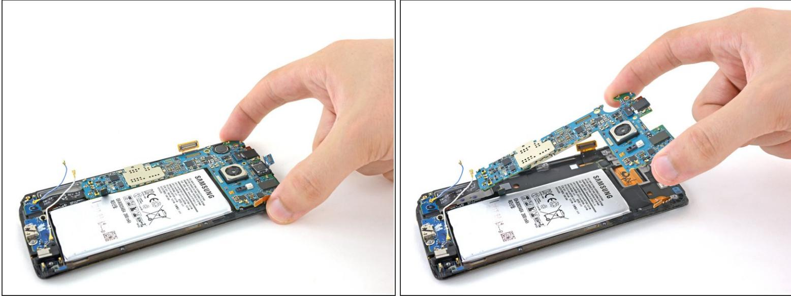
**⚠** The motherboard is an ESD sensitive component and should be handled with care. iFixit recommends using a anti-static bracelet whenever handling components of this nature to avoid damage.
