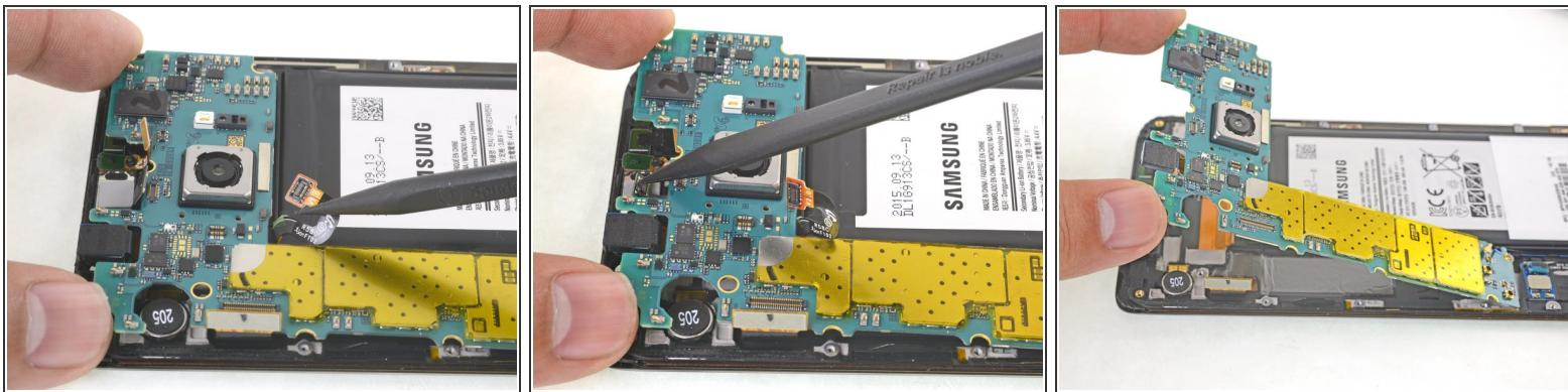
**⚠** Do not lift the motherboard all the way out in this step; the daughterboard ribbon cable on the underside needs to be disconnected first.
