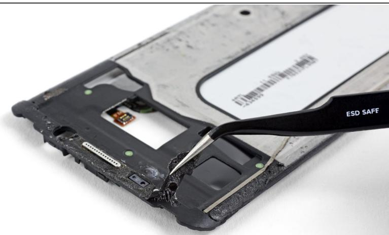
Before installing a new display, it's very important to remove all traces of the old adhesive from the frame, while taking special care to remove any small glass fragments.
