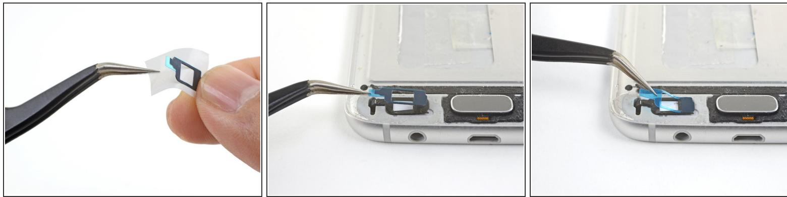
ⓘ This step describes how to replace the capacitive button adhesives. You can skip to the next step if you are not replacing these adhesives.
