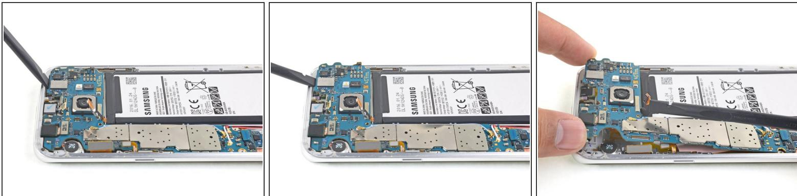
⚠ Do not lift the motherboard out all the way; it is still connected to the daughter board by a cable.
