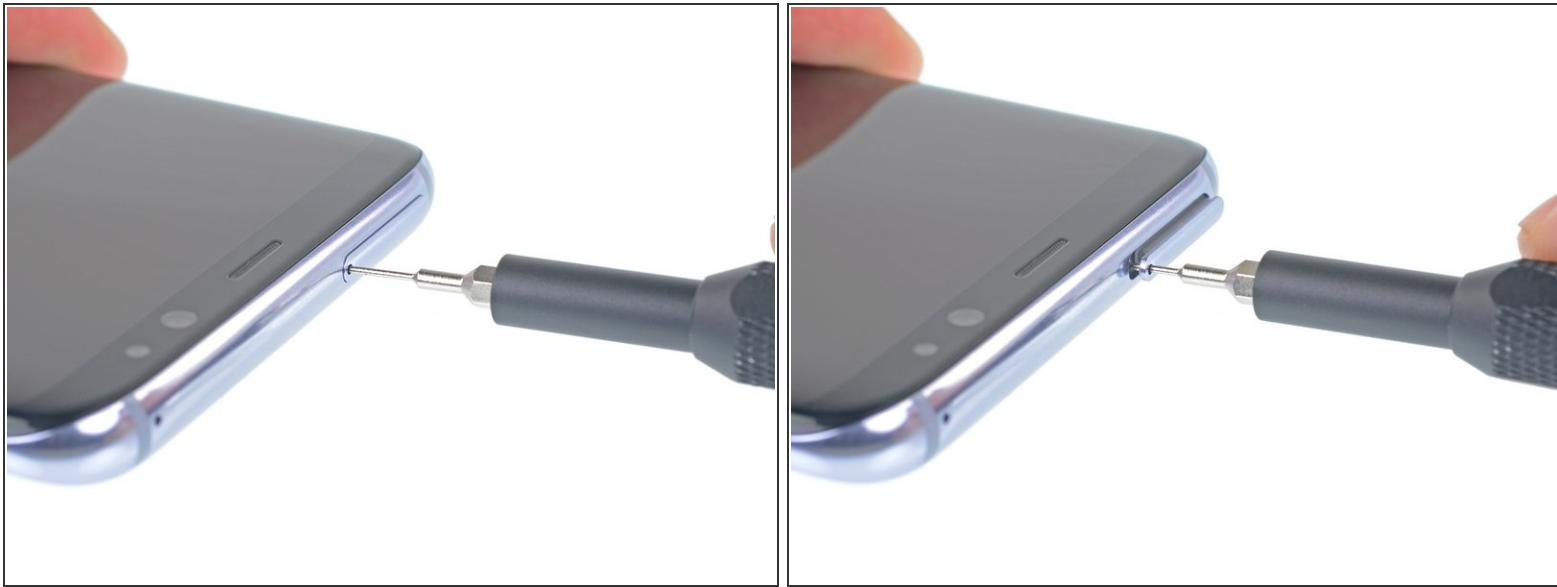
**⚠** The SIM card tray's ejection hole looks almost exactly like the microphone hole, located just a short distance away. Insert your tool only where indicated. Inserting your tool into the microphone hole may result in permanent microphone damage.
