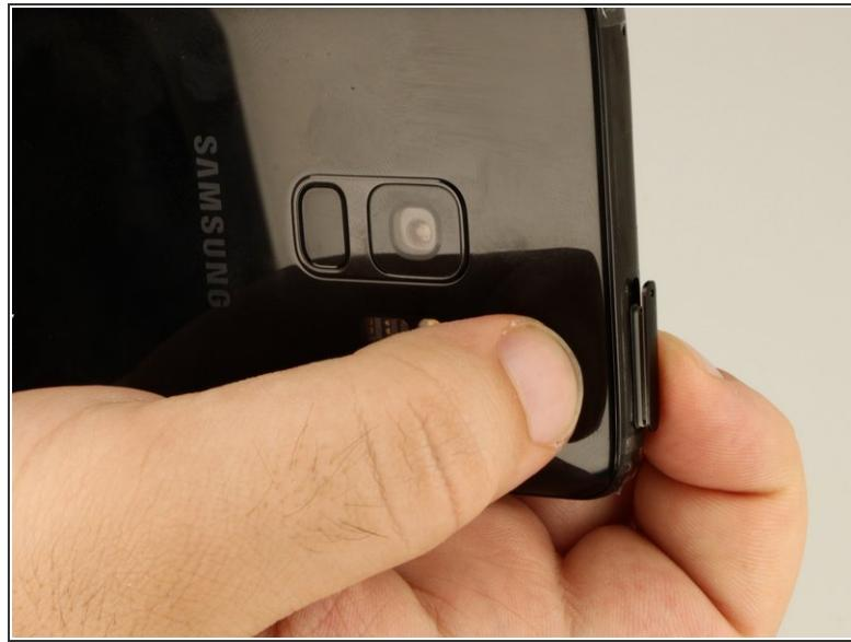
⚠ The SIM card tray's ejection hole and the microphone hole look very similar, be very careful not to insert the tool inside the microphone hole or you might damage the microphone.
