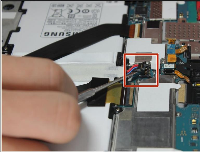
**⚠** When working with electronics, it's important to choose a tool that's ESD-safe to avoid accidental damage to the device. The regular black nylon spudger or a plastic opening tool should be used whenever possible.
