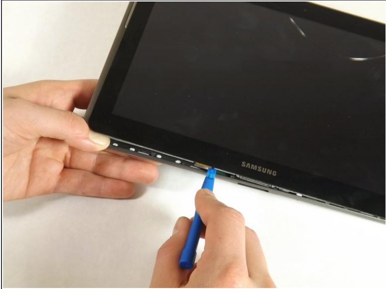
⚠ The plastic opening tool may break during this step. You may need to use the heavy duty spudger instead.
