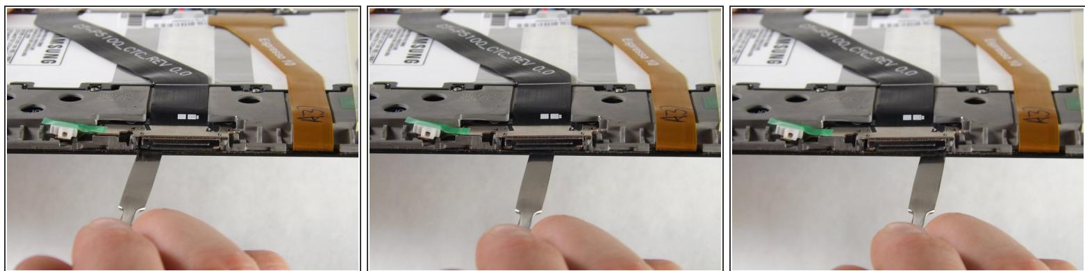
! Be sure to insert the spudger **underneath** the charger port and not inside the charger port to avoid damaging the component
