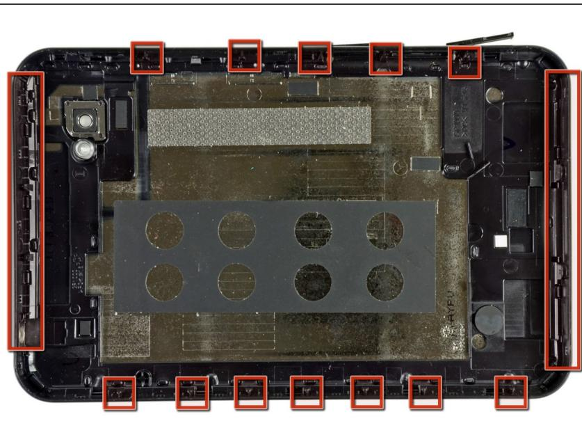
⚠ The following steps will require you to disengage several clips (highlighted in red) around the perimeter of the rear case. The clips are delicate and fragile; proceed with caution.
