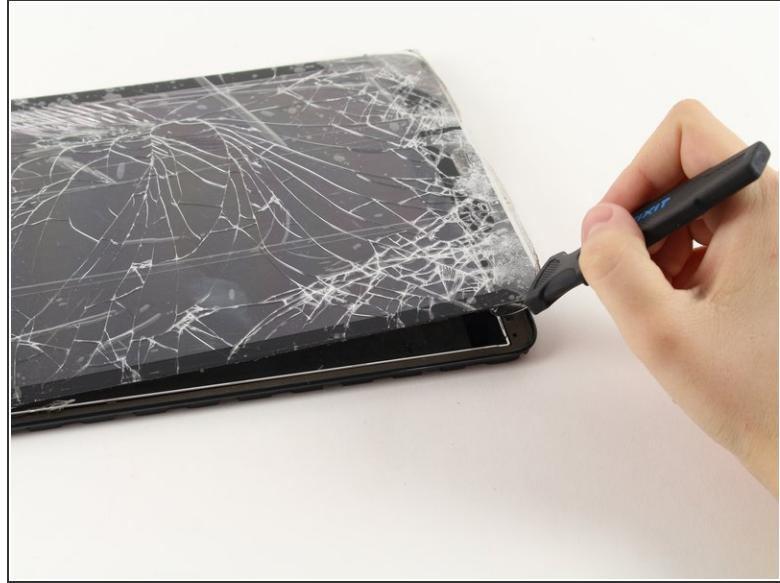
**⚠** The screen may crack during removal, so be wary of broken glass. Apply heat as necessary around the edges of the screen to loosen the adhesive, but be careful not to melt the plastic frame of the tablet.
