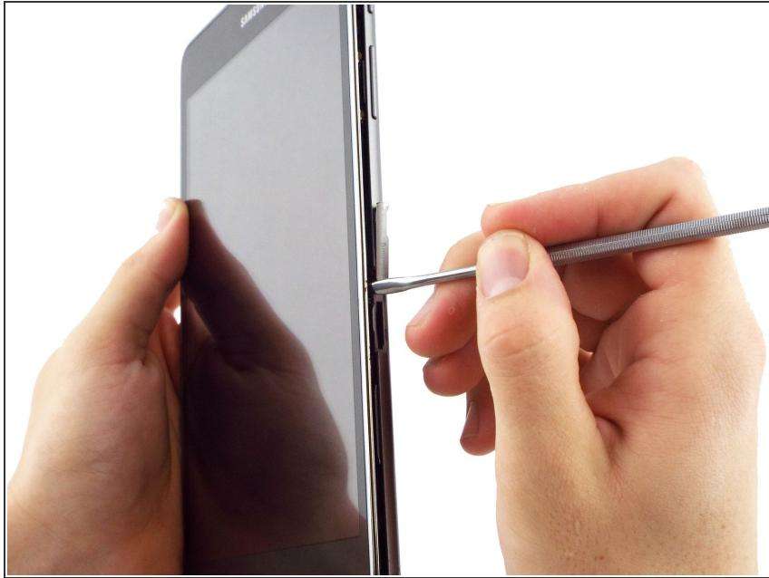
! Make sure the device is turned off before attempting to disassemble it.
