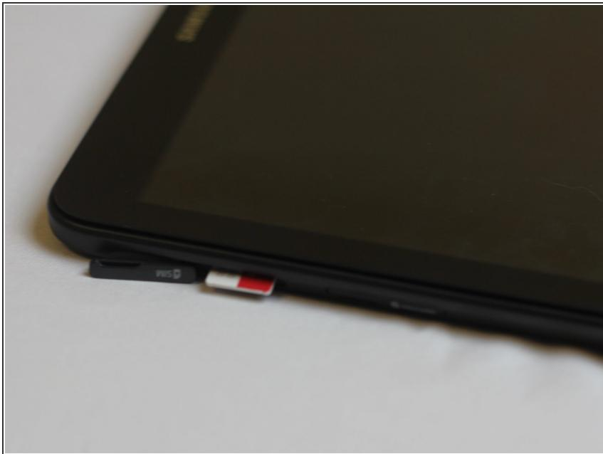
**⚠** If the device has a micro-SD or SIM card inserted, remove them from the device before continuing.
