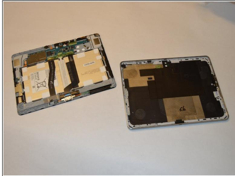
⚠ Be gentle, the front panel is connected to sensitive wiring that may snap if too much pressure is applied.
