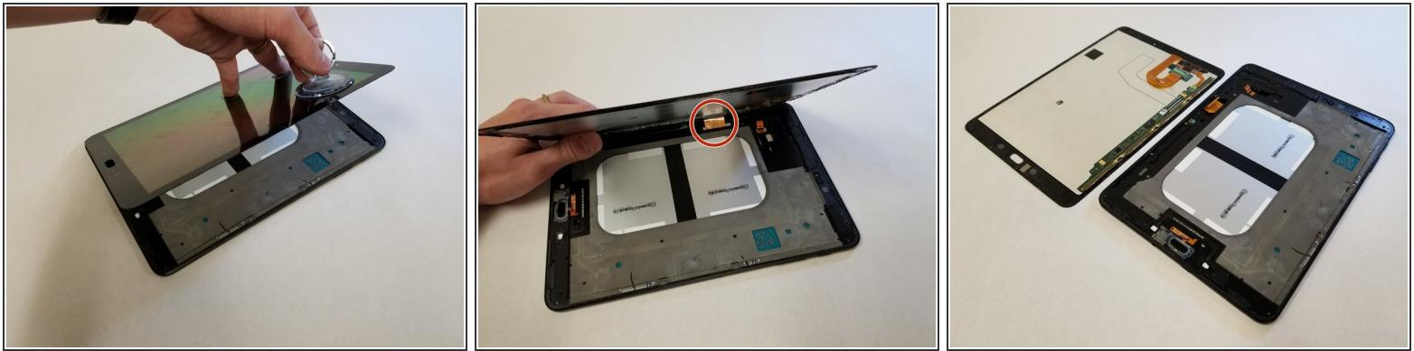
**⚠** As you remove the glass panel, be careful not to tear the ribbon connecting the motherboard to the display.
