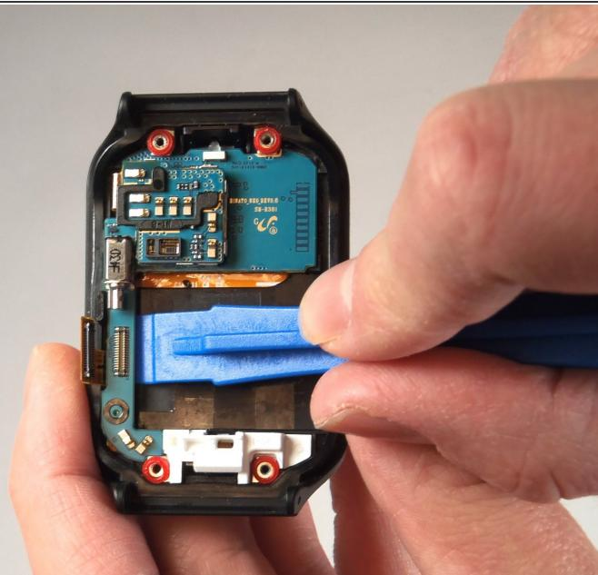
! It is recommended to use antistatic wrist wrap whenever removing the motherboard.
