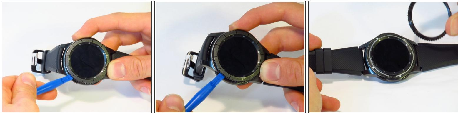
**⚠** Contains small springs and ball bearings. We suggest working over a plate or tray.
