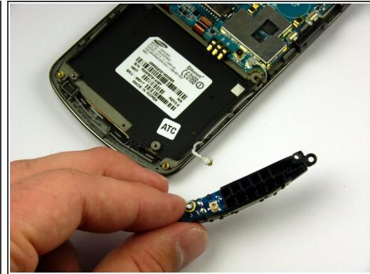
**⚠** There is a wire under the antenna connecting it to the Motherboard. Do not pull off the antenna just yet.
