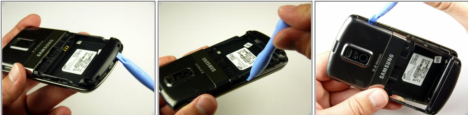
*(i)* The rear case is firmly attached to the phone with clips. Do not be afraid to use a little extra force.
