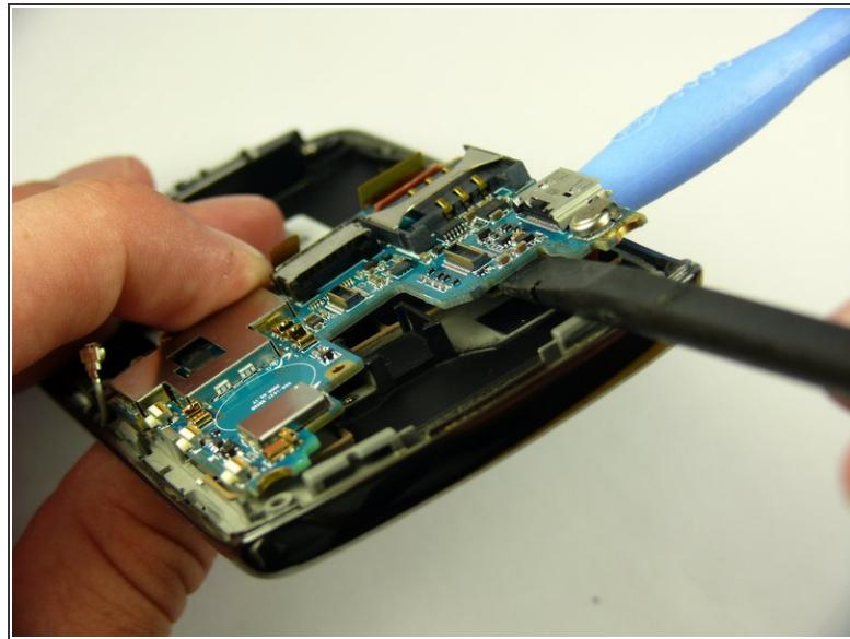
**⚠** There is a ribbon cable under the Motherboard connecting it to the LCD. Do not pull off the Motherboard just yet.
