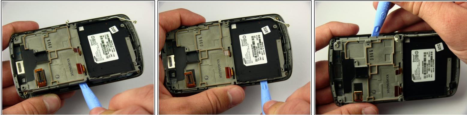
ⓘ The LCD frame is firmly attached to the phone with clips. Do not be afraid to use a little extra force.
