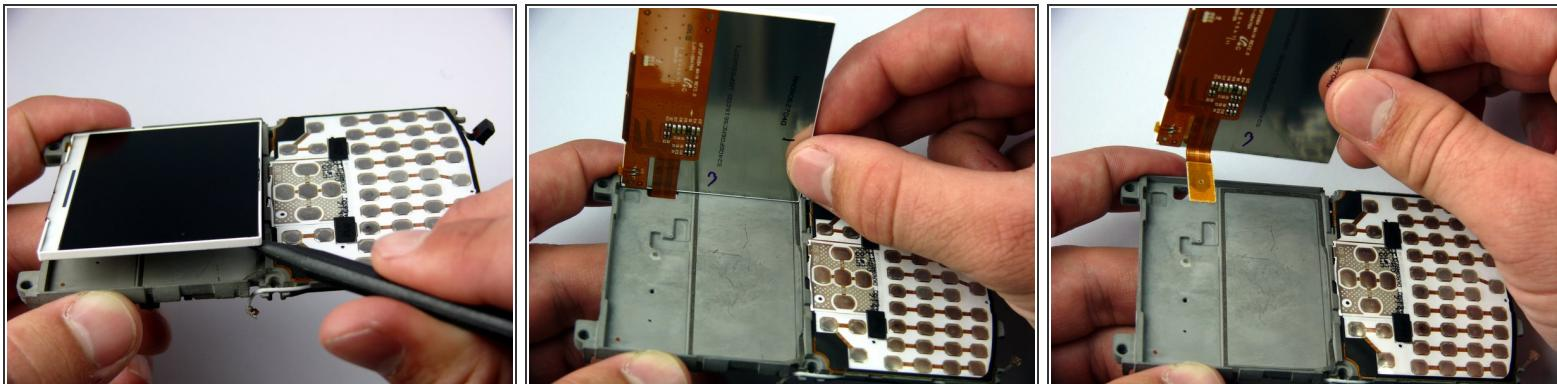
! There is a hanging ribbon cable connected to the LCD screen that passes through the LCD frame.
