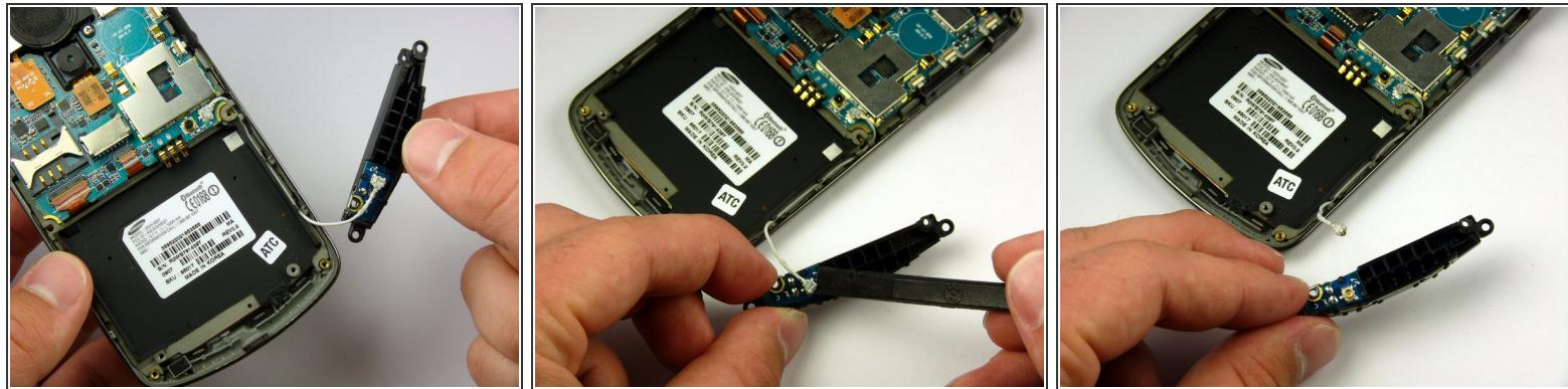
**⚠** There is a wire under the antenna connecting it to the Motherboard. Do not pull off the antenna just yet.
