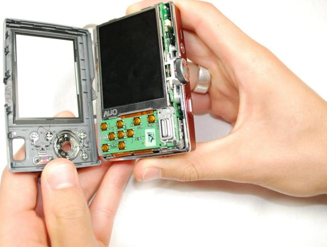
⚠ Carefully pull off the back cover, parts behind the back of the case might fall out.
