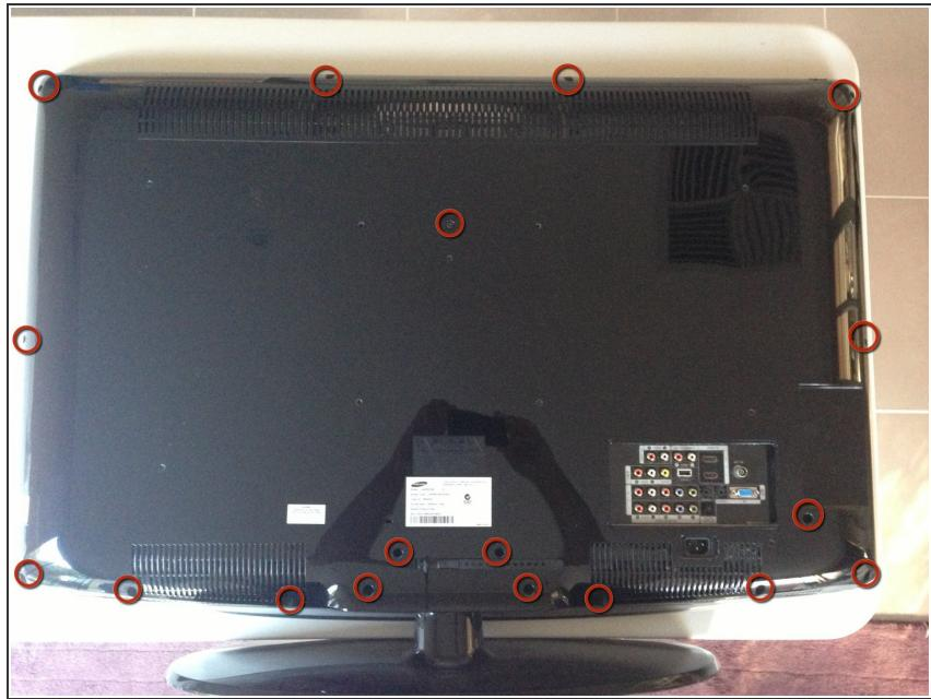
⚠️ Unplug power cable and all AV cables from rear of TV and carefully lay TV face down on a clean flat working surface ensuring that you don't damage the LCD screen.
