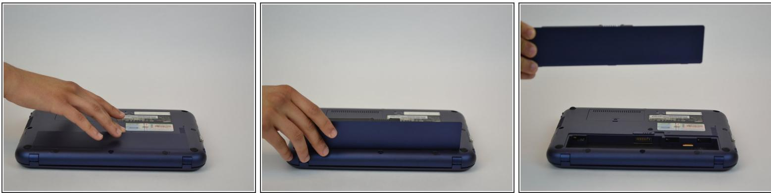
⚠ Make sure the laptop is powered off, and unplugged before removing the battery.
