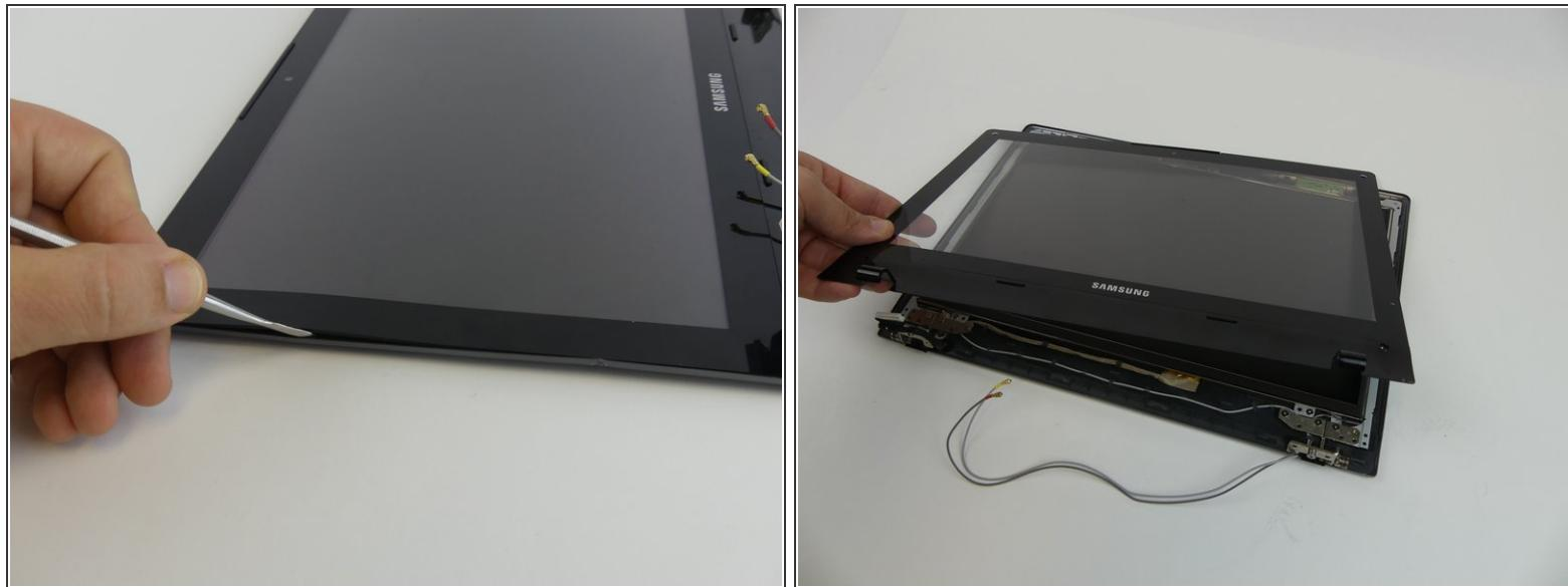
⚠ The metal spudger could scratch the screen.
