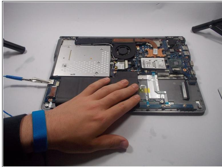
**⚠** All steps following the removal of the back cover should be completed while wearing an Anti static bracelet. This prevents ESD (electrostatic discharge). ESD can damage nearly every part on the inside of your computer.
