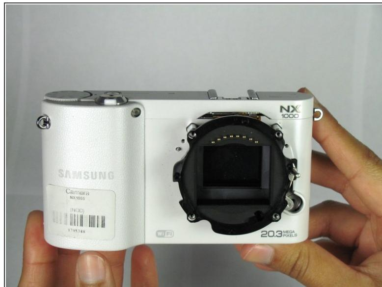
! There are a few loose metal parts and springs. Be careful not to shake the device.
