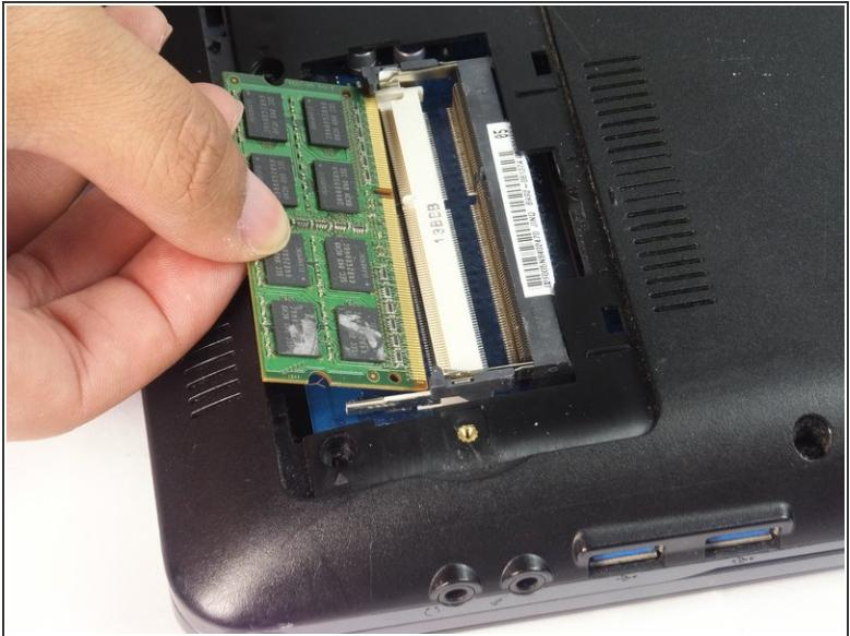
⚠ Carefully slide the RAM away from the slot to remove it.
