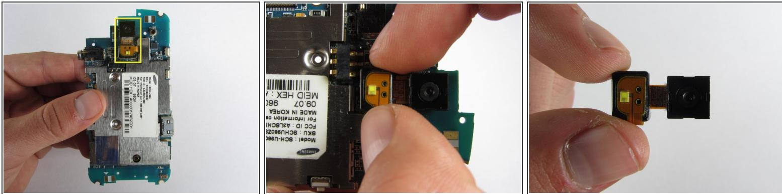
With two fingers carefully detach the camera from the motherboard by lifting straight up.
