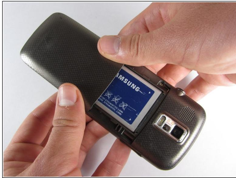
*(i)* Before disassembling your Samsung Rogue, make sure it is powered off.
