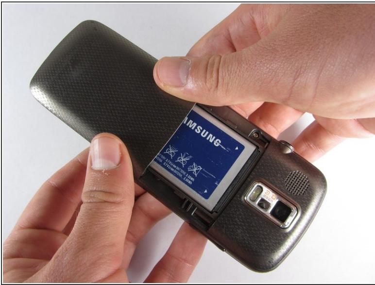
*(i)* Before disassembling your Samsung Rogue, make sure it is powered off.
